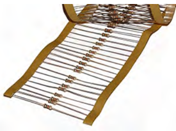
Figure 19.10 Some typical resistors. The color bands indicate the value of the resistance of each resistor.
